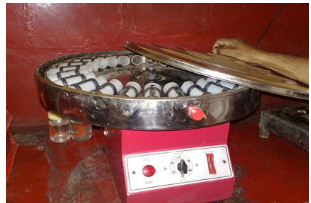
Fig. 5: Centrifugal machine to do the fat test
